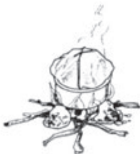
Fig. 4.b: The traditional 3-stone fire
