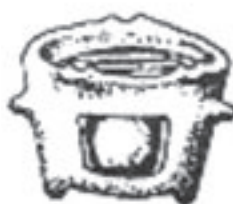
Fig. 5. ee: The all-ceramic stove
