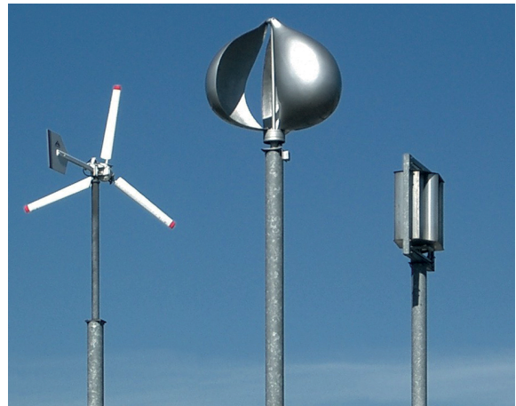
Figure 6: Examples of a small scaled urban wind turbines with vertical or horizontal axis
